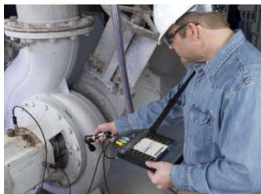
The CSI 2140 Machinery Health Analyzer delivers a single, scalable platform that can perform a variety of machinery health tests. Balancing, temperature trends, and motor diagnostic capabilities coexist with the vibration analysis tools. In addition, single, dual, and four-channel vibration analysis capabilities provide powerful insight into operating condition so you can solve those complex machinery problems.
